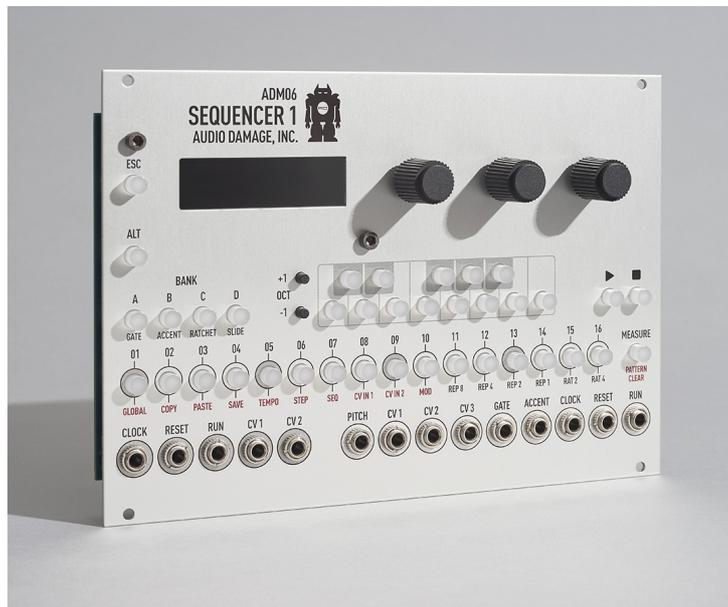
Sequencer 1 is a top-of-the-line x0x-flavored Eurorack sequencer, for controlling up to four voices at once.
