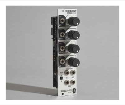
Dimensions is a true stereo chorus effect for the Eurorack modular system featuring two algorithms. The first is a direct port of our Fluid chorus plug-in, and the second is taken from the unit's namesake. With automatic routing based upon what you plug in the I/O, Dimensions can do mono->mono, mono->stereo, and true stereo chorus duties.
