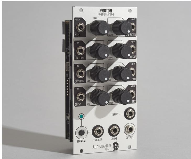
Proton is Audio Damage's take on the classic Karplus-Strong tuned delay line physical modelling synthesis. Take a capable "vintage digital" style delay line with 1V/Oct clocking, and add an enveloped noise burst, and you have a plucked string physical model. We wrap this up in some of our standard Audio Damage aural hijinks, and Proton is the result.
